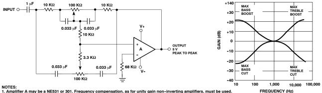
Amplifier A may be a NE531 or 301. Frequency compensation, as for unity gain non-inverting amplifiers, must be used.
