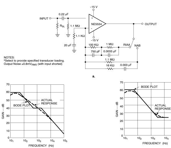
b. Bode Plot of RIAA Equalization and the Response Realized in an Actual Circuit Using the 531.
