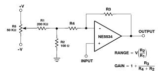
Figure 23. Universal Offset Null for Non-Inverting Amplifiers
