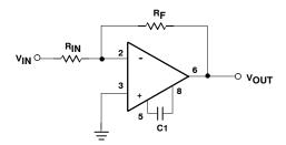
Figure 11. Unity Gain Inverting Configuration
