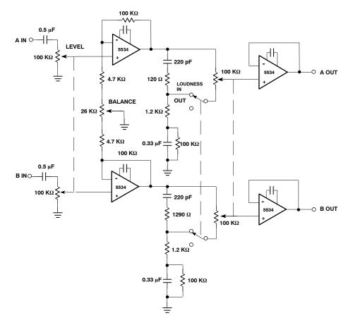
Figure 21. Balance Amplifier with Loudness Control
