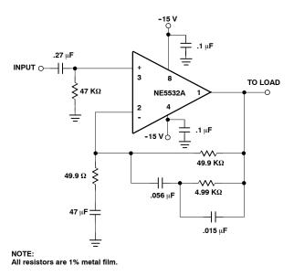
Figure 3. RIAA Phonograph Preamplifier Using the NE5532A
