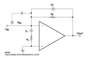
Figure 12. External Compensation for Wideband Voltage Follower
