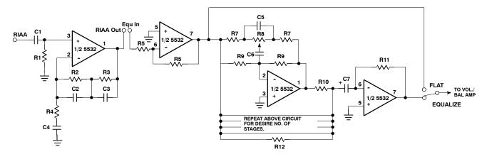
Figure 1. RIAA - Equalizer Schematic
